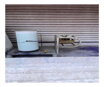
A thermograph is an instrument that records air temperature continuously on graphing paper. It usually consists of a cylinder made to revolve once each week by means of a clock working inside. A sheet of graph paper is fastened on the outside.
