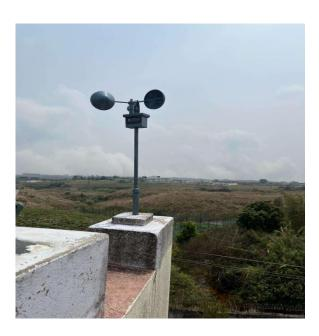
An anemometer is an instrument that measures wind speed and wind pressure. Anemometer are important tools for meteorologist who study weather patterns.
