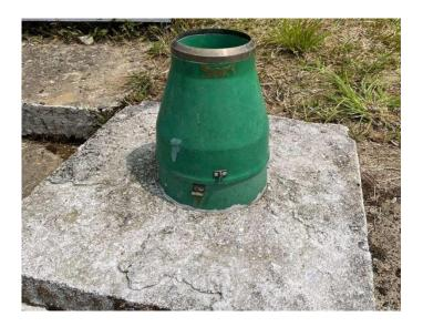
A rain gauge is a meteorological instrument to measure the precipitating rain in a given amount of time per unit area. The instrument consists of a collection container which is placed in an open area. The precipitation is measured in terms of the height of the precipitated water accumulated in the container per given time and is expressed in millimetres.
