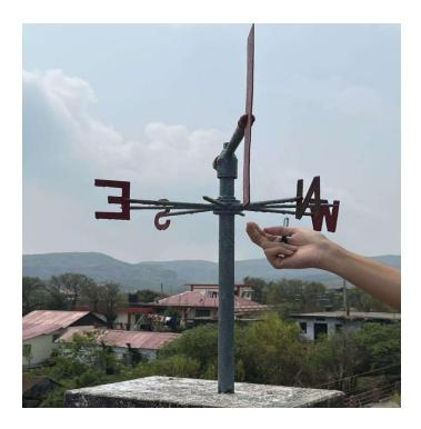
A wind vane is a device that measures the direction of the wind. The wind vane is usually combined with the anemometer. Wind direction is the direction from which is blowing.
