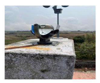
A device in which a glass sphere concentrates the Sun's rays on to a calibrated paper where the resulting burns register the time and duration of sunshine. The instrument must be pre-set for a given latitude. This type of recorder has been in use since about 1880.
