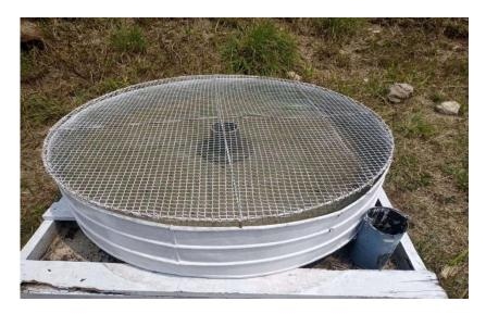
Pan evaporation is a weather measurement system that integrates several climatic conditions including rainfall, humidity, solar-radiation wind temperature and drought dispersion. The system distinguishes the rate of evaporation based on the weather factor.
